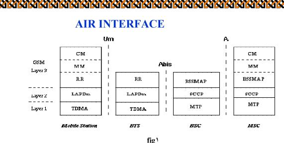
Signaling protocol structure in GSM
