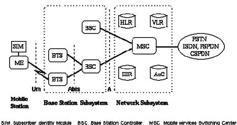
ME Wobile Equipment HLR Home Location Register EIF Equipment Identity Register BTS Base Transceiver Station VLR Visitor Location Register AuC Authentication Certer
